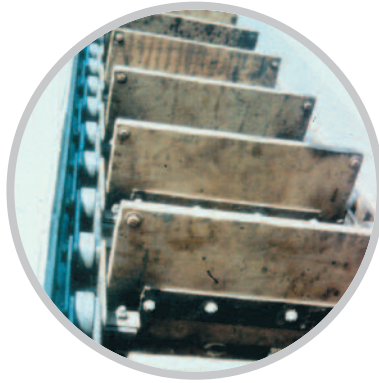
Conveyor Chain with scraper attachments handling fishmeal products in Peru.
