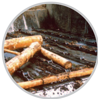
Renold Special Chain designed for log elevators, used here in a paper pulp plant, processing 1200 tonnes of timber per day.
