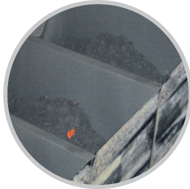
Special Double Strand Conveyor Chain is designed to give an enhanced chain life in the hot and dusty conditions of a Cement Clinker.
