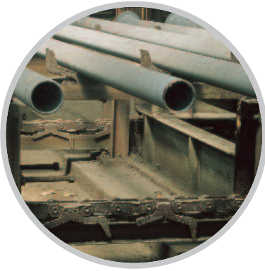
Two strands of special conveyor chain delivering spun cast iron pipes.
