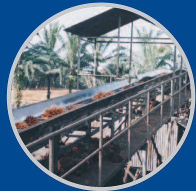
Palm Oil Mill scraper conveyor - Palm Oil is extracted from the bunches of fruits and the waste is conveyed away.
