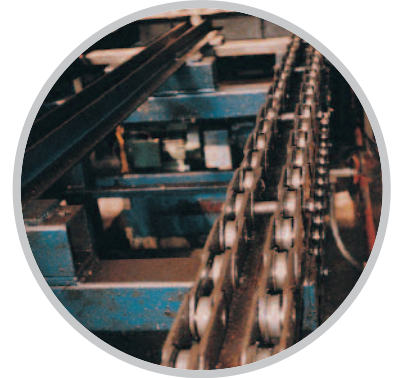
Special Double Strand Conveyor Chain used in a corrugated roofing plant in Chile.
