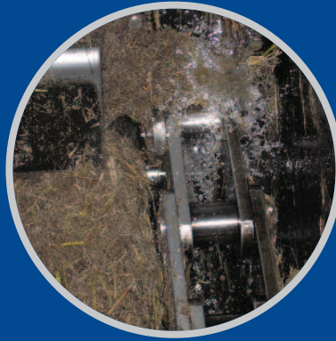
Heavy duty conveyor chain operating in sugar industry.
